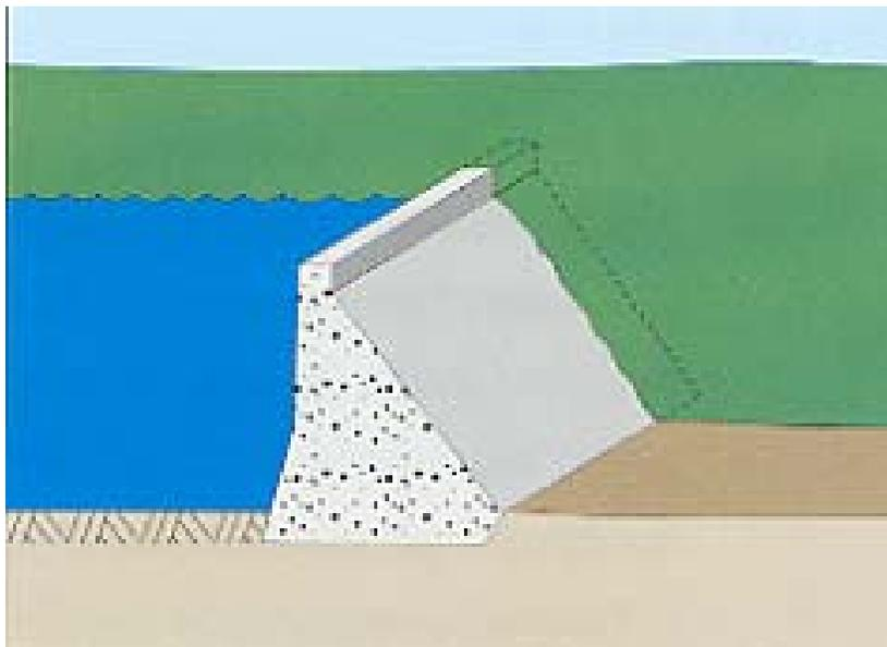
Gravity dams are constructed of vertical blocks of concrete with flexible seals in the joints between the blocks.
