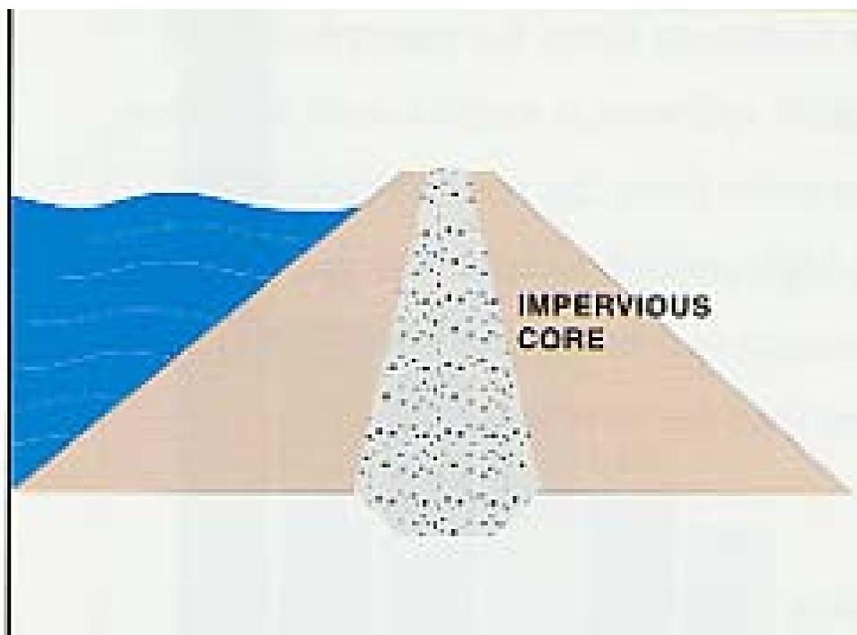
Materials used for embankment dams include natural soil or rock, or waste materials obtained from mining or milling operations. An embankment dam is termed an “earthfill” or “rockfill” dam depending on whether it is comprised of compacted earth or mostly compacted or dumped rock.
